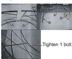
Attach two parts of Arch (B) to top Arch (A) as shown in figure.
